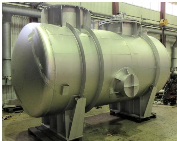
Horizontal External Pump Tank
