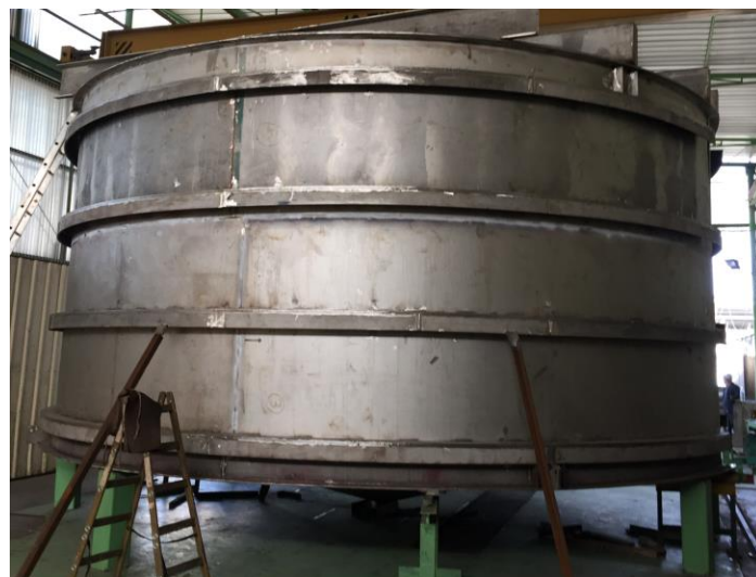
Vertical External Pump Tank
