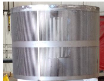
Acid Tower Internal Strainer
