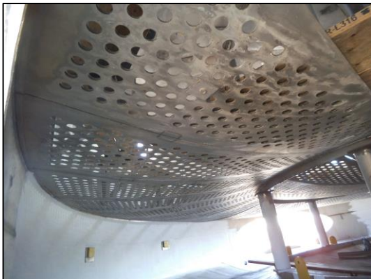
Catenary shaped catalyst support plates
