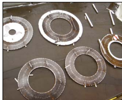
Heat Exchanger Baffle Plates
