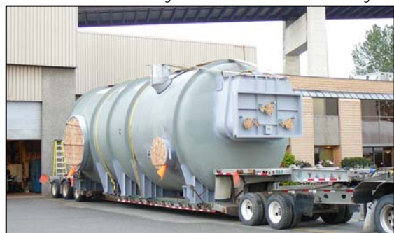
NORAM Sulphur Furnace
