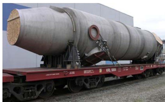
Radial Flow Stainless Steel Gas-to-Gas Heat Exchanger
