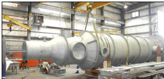
NORAM Split Flow Preheater Exchanger
