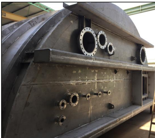
NORAM Acid Pump Tank Fabrication
