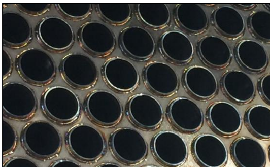
NORAM Gas Exchanger with Hot Sweep Tube Bundle
