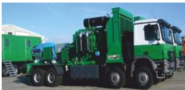
Frac Pumping Unit
