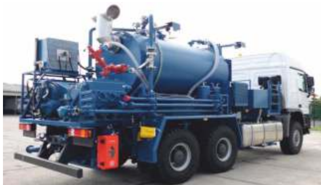
Hot Oil Pumping Unit
